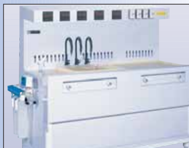
Overhead control panel eliminates the need to reach over process tanks.
