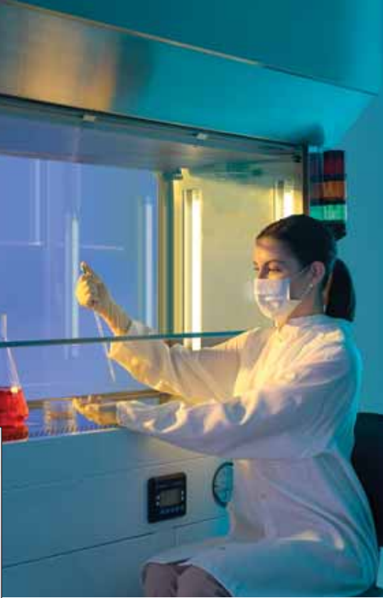
Electronic interlocks and status lights ensure access from one side only.
