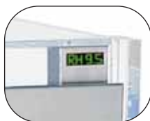
Miniaturized LED monitors humidity and displays set point
