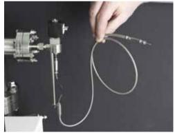
Micro-flow capillary inlet. Sampling rate 12 μl/min. Single or multi-capillary inlet option.
