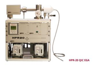
The Hiden HPR-20 QIC EGA gas analysis system is configured for continuous analysis of evolved gases and vapours from thermogravimetric analysers (TGA). Interface systems are available for most TGA instruments. The TGA interface includes re-entrant furnace sampling, providing close coupling to the TGA furnace region for optimized evolved gas/vapour analysis.
